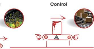
Checkweighing & sorting Weighing for the grading of products or missing parts check before shipment.
